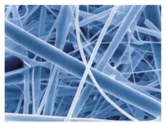
Fig. 5 Thermally embossed micro-glassfiber paper 5 µm
