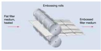
Fig. 9 Thermal embossing process
