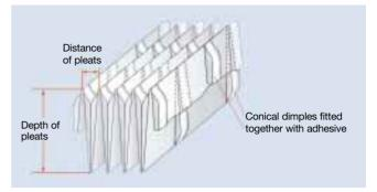
Fig. 10 Thermal embossing technique: no additional spacing materials
