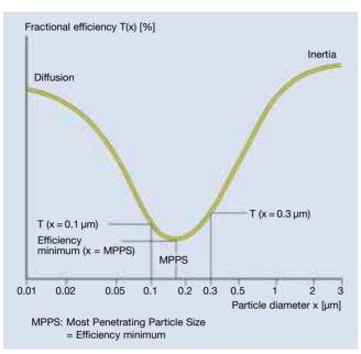
Fig. 2 Minimum curve of a HEPA filter medium
