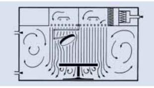
Fig. 4a Operation theater with low-turbulence displacement flow over operation table, HEPA filters in the air duct
