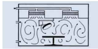
Fig. 3 Operation theater with turbulent mixed ventilation
