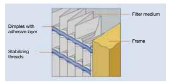
Fig. 11 Thermal embossing technique
