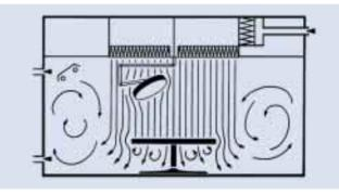
Fig. 4b Operation theater with low-turbulence displacement flow over operation table, HEPA filters in the ceiling
